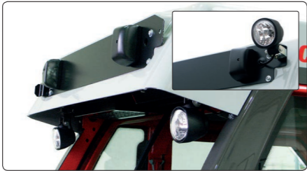
One or two working lights on or below the cab roof provide best view of the rear working area.
