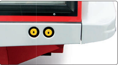
The exterior electric control for the front linkage is standard and makes mounting of attachments much easier.
