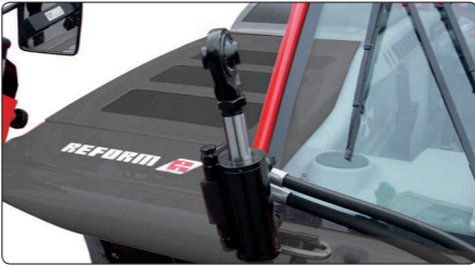
With the hydraulic top link , you can react to uneven ground quickly from the cab or adjust the cutting height with the push of a button.
