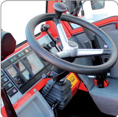
The tilt-adjustable steering column ensures an optimum seating position.
