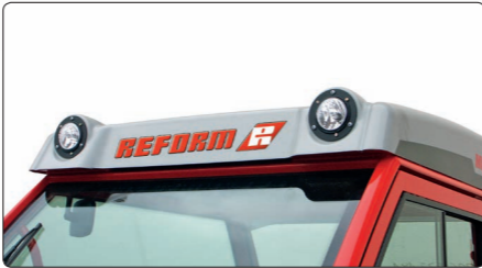
The integrated auxiliary lights (optionally also in LED) at the roof front ensures maximum visibility, turning night virtually into day.
