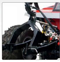
The Metrac H4 X has a **front linkage** with integrated lateral displacement.
