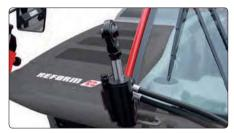
With the **hydraulic top link**, you can react to uneven ground quickly from the cab or adjust the cutting height with the push of a button.
