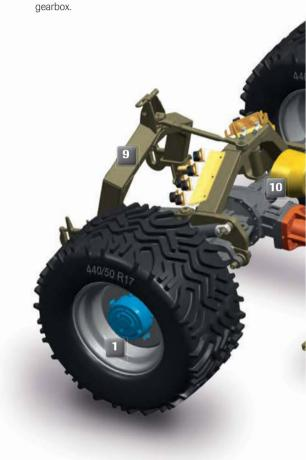
Central joint and oscillating axle
