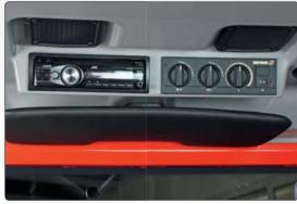
A **stereo radio with CD** will make your workday even more enjoyable (option). The **roof area** also accommodates the controls for the air conditioning and ventilation system, switches for auxiliary lights, the cab illumination, as well as rear view mirror and sun visor.
