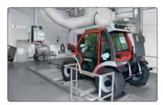
Before delivery, all vehicles undergo intensive **functional testing** such as here on the roller test hed
