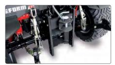
The height adjustable **trailer hitches with slide** are a special advantage (mechanical, automatic, or with ball head).
