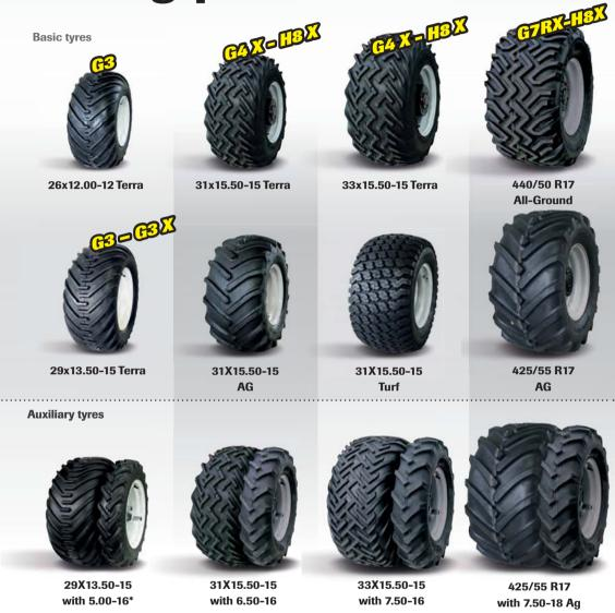
The wide low-pressure tyres with various special profiles ensure **maximum traction**, low ground pressure and reliable turf protection. They provide grip on difficult soils and on steep slopes.
