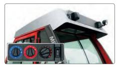
Comfortable climate with roof-integrated **air conditioning** or additional fresh air supply for closed cab with the integrated **roof ventilation system** (not with G7 RX/ H7 RX).
