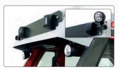
One or two **working lights** on or below the cab roof provide best view of the rear working area.
