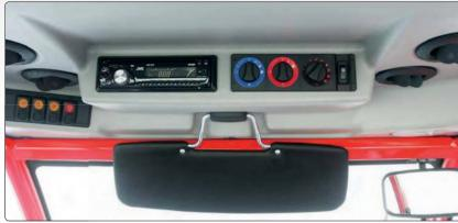
A **stereo radio with CD** will make your workday even more enjoyable (option). The **roof area** also accommodates the controls for the air conditioning and ventilation system, switches for auxiliary lights, the cab illumination, as well as rear view mirror and sun visor.
