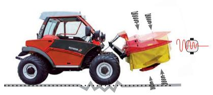
The impact load is minimised by gas pressure accumulators.
