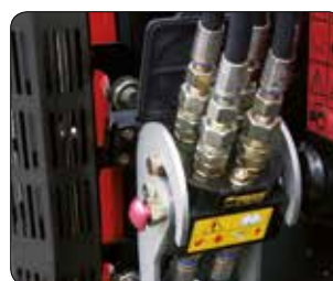
Multi-hose coupling Quick and hassle-free coupling of the hydraulic connectors.
