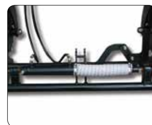
Hydr. tool lock Quick mounting and removing of attachments without leaving the cab.
