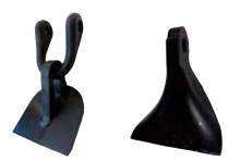
High tempered "M"-Hammer flails to ensure clean cut and maximum shredding using less power forged from special steel with double reinforced rib to make it more fracture proof or alternatively a rotor with "M"-Shackle flails to cope with stones or other debris (MU-H + H/S,
