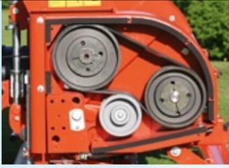
The continuous crankshaft is driven on both sides by „elastic“ ribbed V belts. The maintenance-free drive is encapsulated and protected against dust and dirt.
