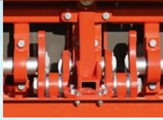
The extremely sturdy, computer-optimised crankshaft runs on large sized ball bearings. Precisely calculated counterweights allow for the TERRA SPIKE® XF/XD unrivalled smooth running.
