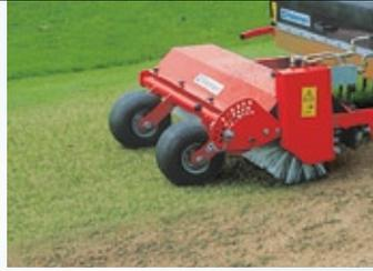
If the optional hydraulic rotary brush is used instead of the rear roller, the turf is first top-dressed and then deep loosened while the top-dress material is brushed into the turf. This reduces the number of passes.
