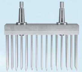
Solid tines 5 x 65, 5 x 135, 8 x 65 or 8 x 150 mm are mounted in the multi-tine holder "nail board". 24, 16 or 8 tines can be mounted, depending on the task and the required hole pattern. The "sandwich construction" of the nail board allows quick and easy tine replacement.
