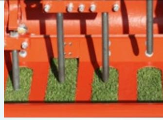
The optional turf retainer prevents damage to shallow rooted turf.
