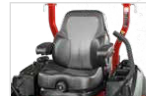
Premium High-back Suspension Seat Seat with adjustable suspension, padded arm rests and fore- and aft positioning.
